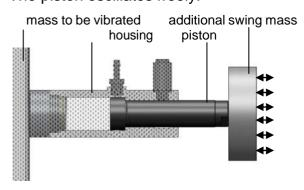
In some types the weight of the piston and the housing differs only marginally. In these cases the data for the freely oscillating piston is given with a usual swing mass SM (**SW 3**). The designation of the swing mass SM is given in brackets (P + SM 8-2; i.e. piston P plus swing mass SM 8-2).
